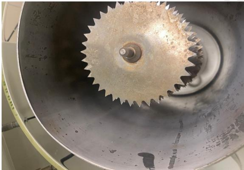
Figure 3: Buchi Spray Dryer Particle Collector showing particle sticking
