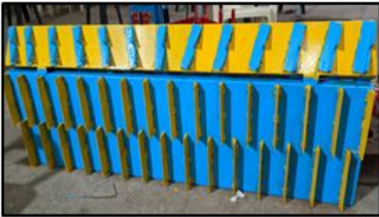
Fig. 6 Blade arrangement on developed clod crusher
