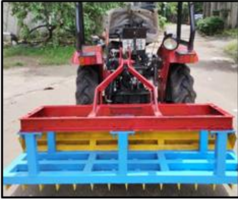
Fig.5 Fabricated mini tractor-operated clod crusher
