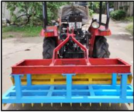
Fig.5 Fabricated mini tractor-operated clod crusher
