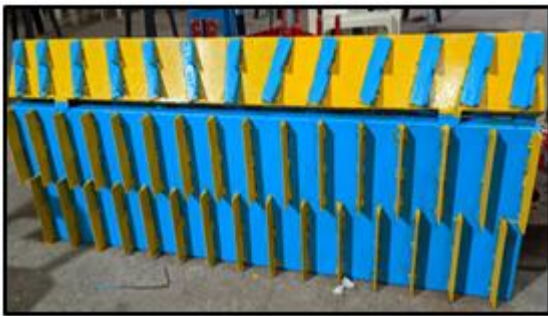
Fig. 6 Blade arrangement on developed clod crusher
