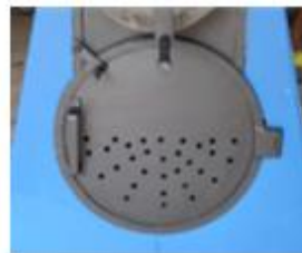
Fig. 2 Semi-perforated door of combustion chamber
