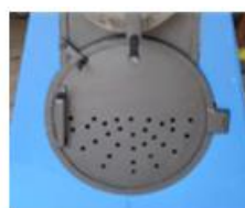
Fig. 2 Semi-perforated door of combustion chamber
