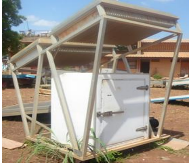
Figure 1: Photo of the adsorption solar refrigerator
