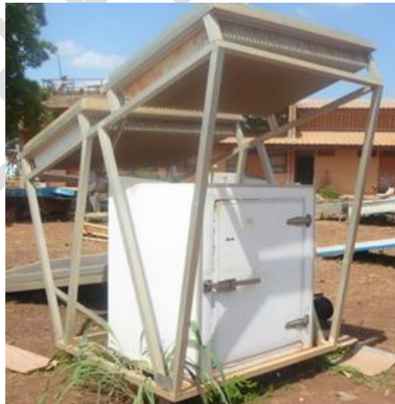
Figure 1: Photo of the adsorption solar refrigerator
