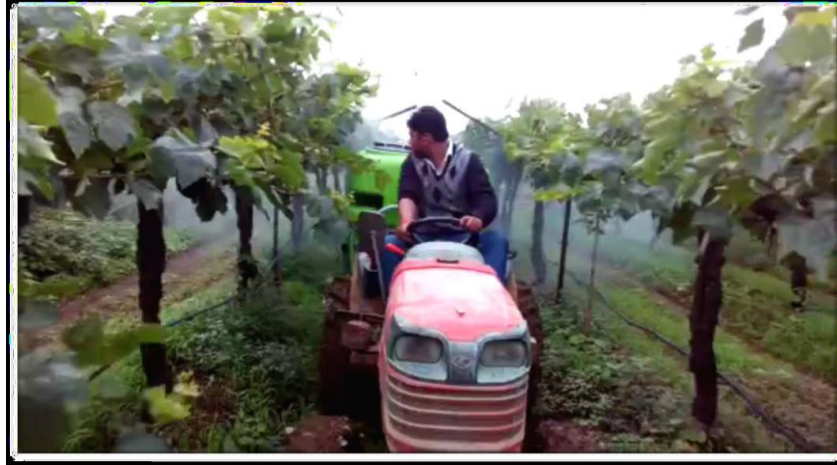
Plate 4. Field evaluation of axial flow blower with air assisted orchard sprayer (Grapevineyard)
