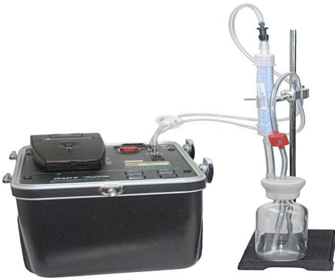
Figure 1: Setup of RAD-7 for radon measurement in water [13]
