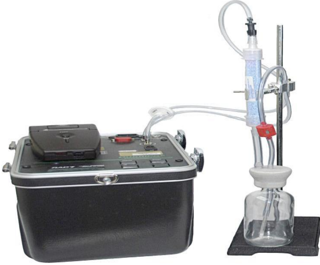
Figure1: Setup of RAD-7 for radon measurement in water(DURRIDGE, 2020)
