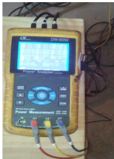
Fig. 1. Lutron 3 Phase digital Power Analyser/meter
