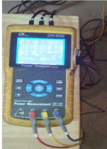
Figure 1. Lutron 3 Phase digital Power Analyser/meter
