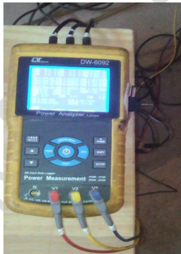
Figure 1. Lutron 3 Phase digital Power Analyser/meter
