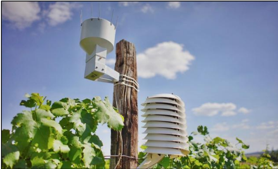
Figure 9: Automated weather observing system
