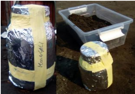
Figure 3: Conditioning of soil samples polluted by hydrocarbons for transport to laboratory
