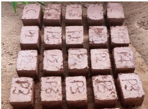
Fig.3. Photograph showing freshly moulded block specimen
