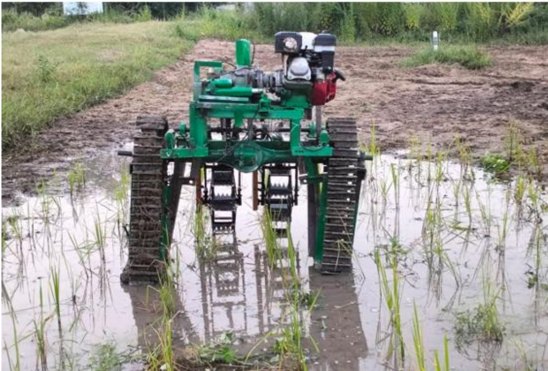
Plate 1: Front view of developed remote operated paddy weeder
