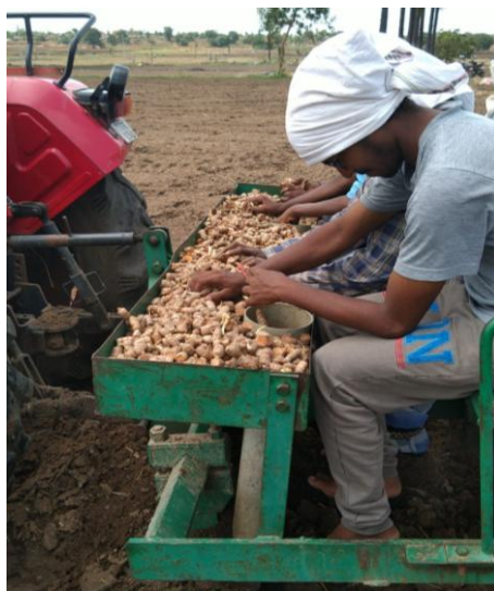
Fig. 2 Semi-automatic planter's turmeric seed rhizome planting
