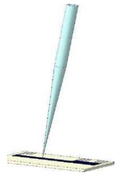
Figure 6. Mutual arrangement of sample and microcontact in microcontact spectroscopy
