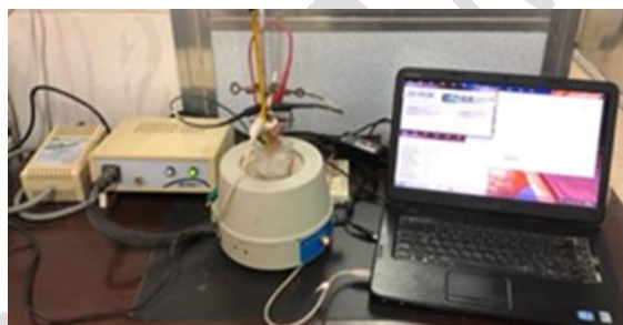
Fig. 1: setup of cyclic voltammetry
