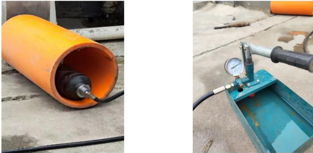
fig7.Pressure test of ballast tank
