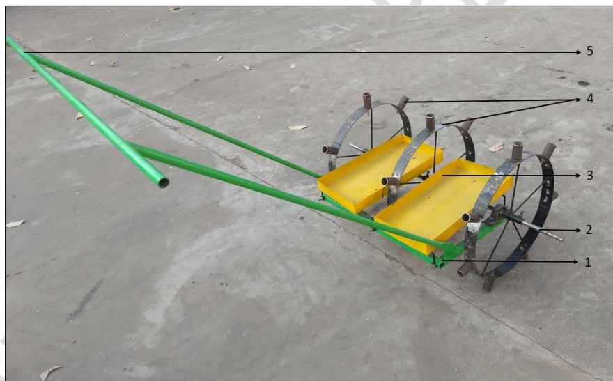
1.Frame; 2. Shaft; 3. For loads; 4. Dibble wheels with lugs; 5. Handle
