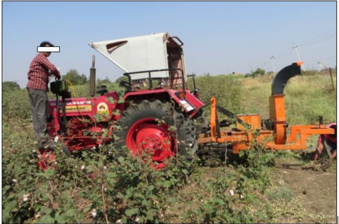
Plate 7. Measurement of fuel consumption of cotton stalk shredder cum uprooter
