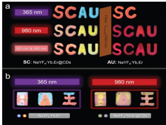
Figure 8(a,b) shows the luminescent anti-counterfeiting application patterns of NaYF 4 :Yb,Er@CDs nanocomposite material and NaYF 4 :Yb,Er phosphor.
