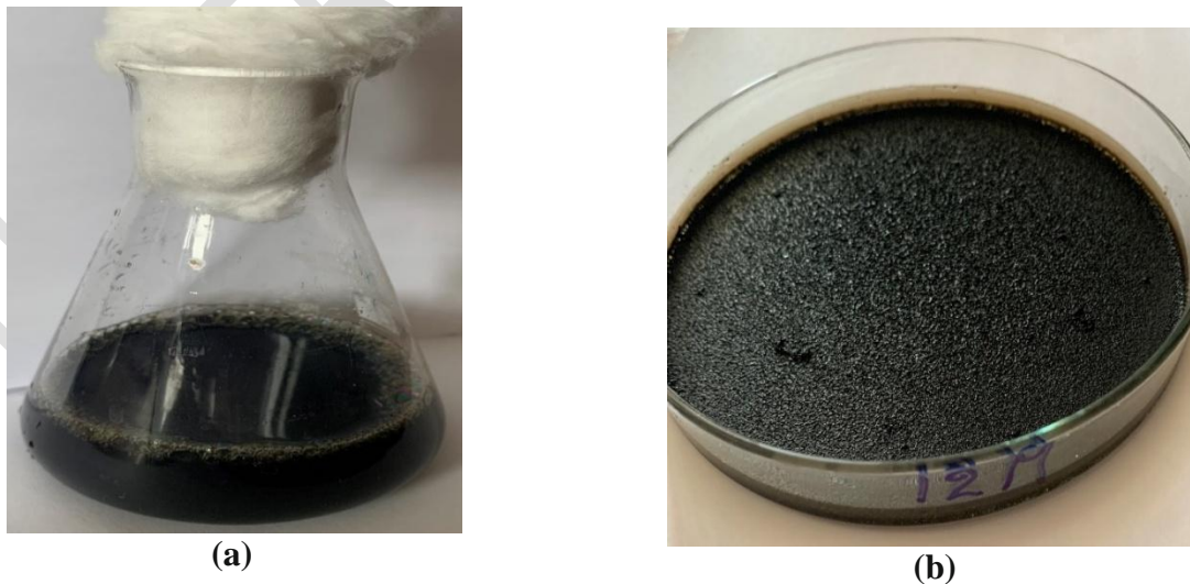
Figure 17. (a). Pigment extracted by ethanol solvent; (b). Dried pigment after ethanol extraction
