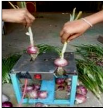
Fig .3: Battery operated onion root and shoot cutting machine
