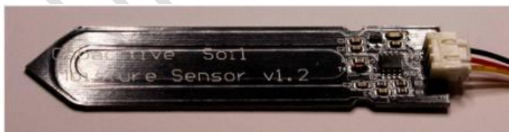
Fig 3. "Capacitive" soil moisture sensor, showcasing a coplanar concentric capacitor design.
