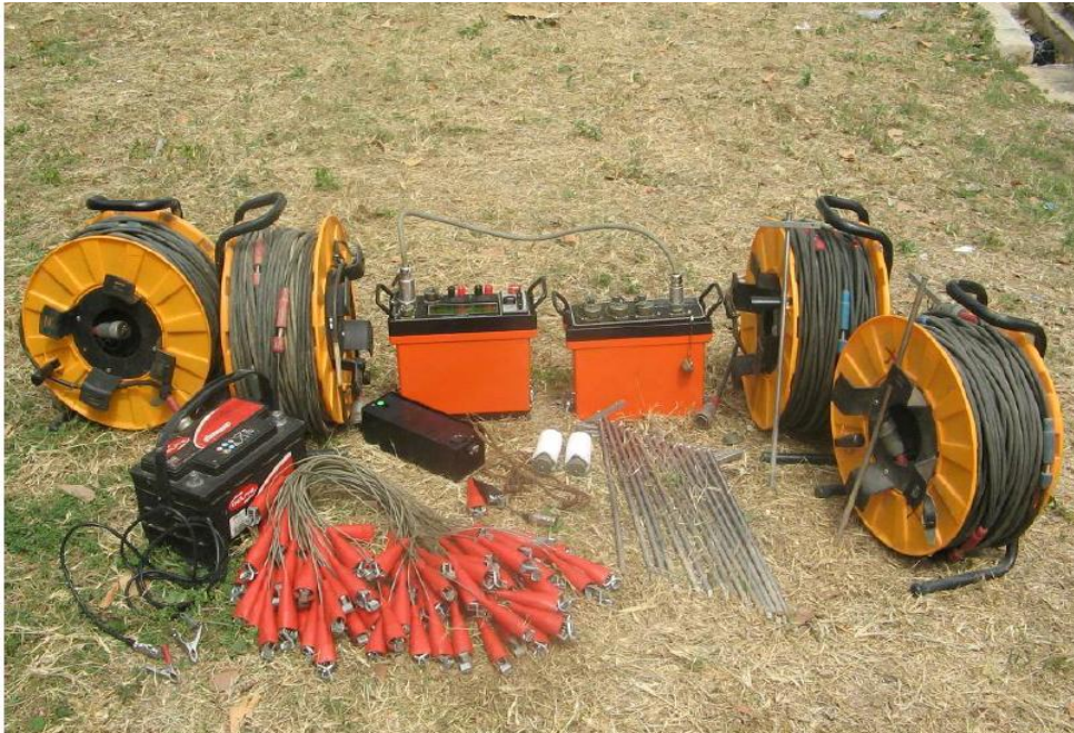
PLATE 1: Electrical resistivity equipment and other accessories.
