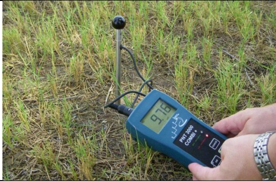
Fig. 3 Direct measurement of soil salinity using salinity probe
