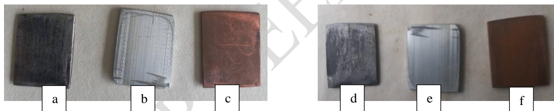
Figure 4: Metal samples before and after corrosion test
