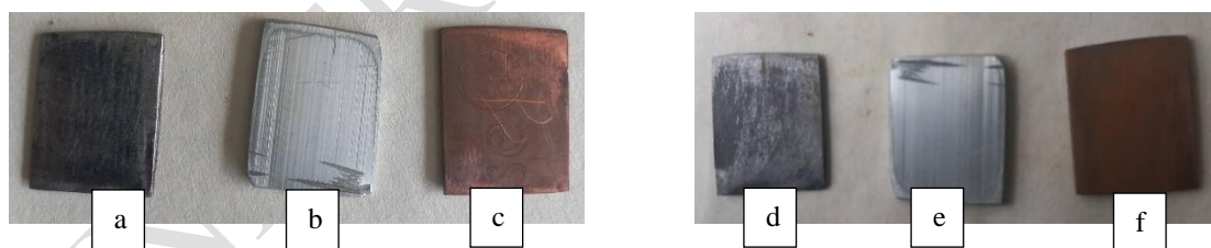
Figure 4: Metal samples before and after corrosion test
