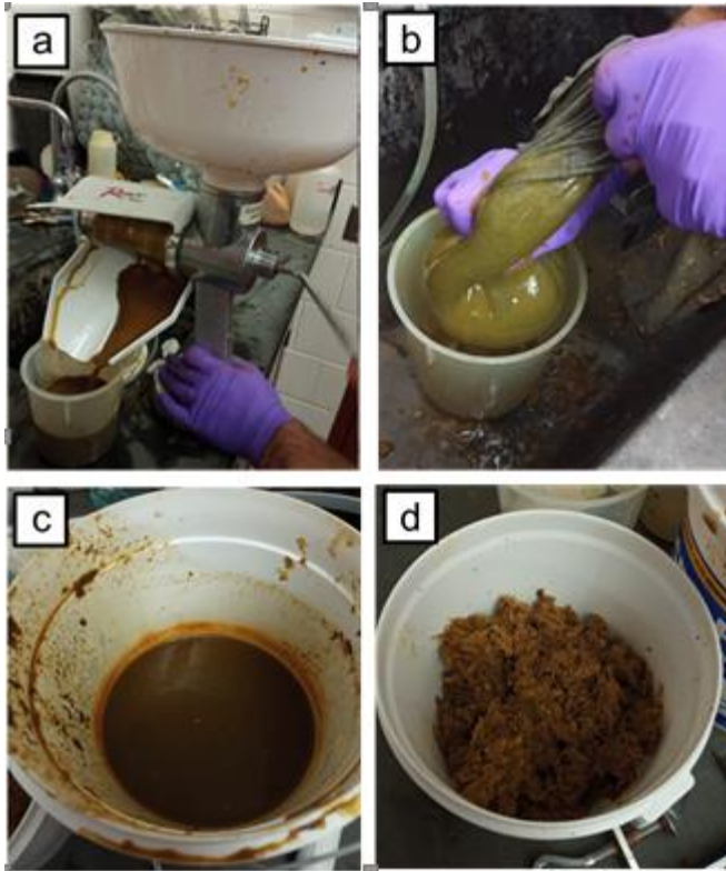
Fig. 4: Laboratory Manure Dewatering, a) Laboratory Screw Press, b) T-shirt, c) Liquid Manure Effluent, d) Solid Manure Effluent [25]
