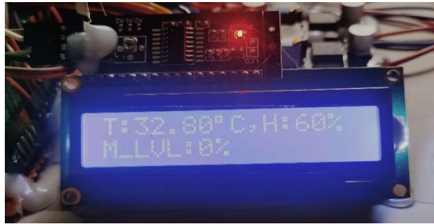
Fig.11 Monitor Sensor data via LCD
