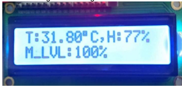
Fig.9 Monitor moisture Sensor data via LCD.
