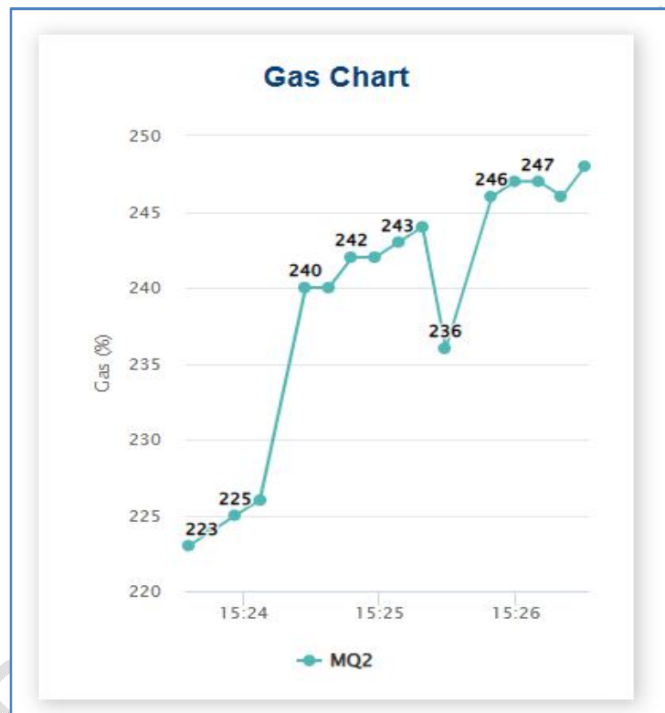
Fig. 7. Real-time measurement of smoke concentration in the air from the dashboard display
