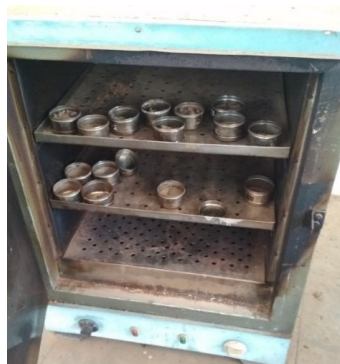
Fig. 1. Soil moisture content measurement by oven drying method
