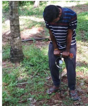
Fig. 3. Soil cone index measurement by cone penetrometer
