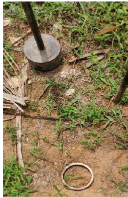
Fig. 2. Soil bulk density measurement by core cutter method
