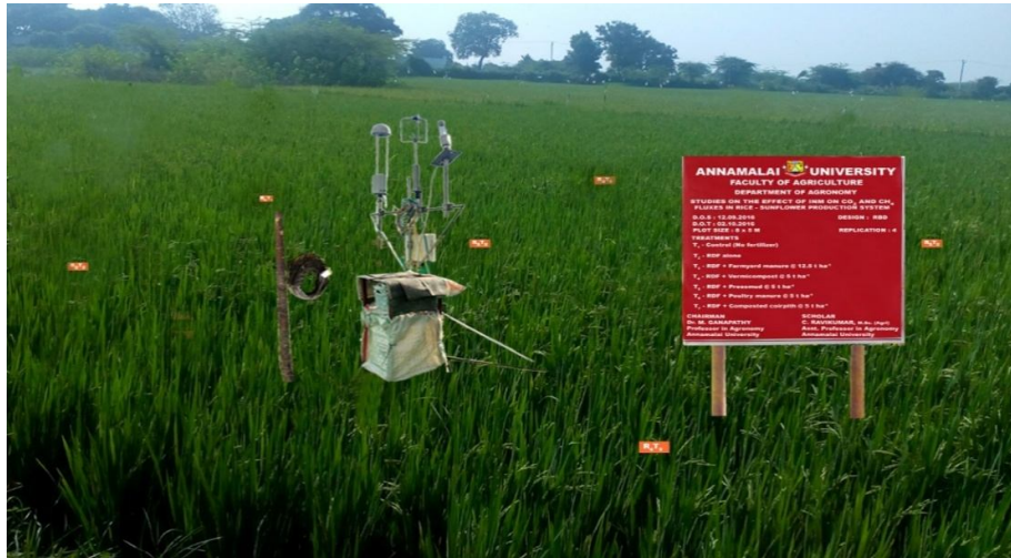
Fig.1 LICOR CH 4 and CO 2 Analyzer
