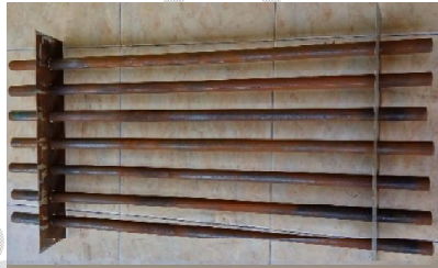
Fig. 1. Design of a one-pass heat exchanger made of black steel, with a total of 7 pipes
