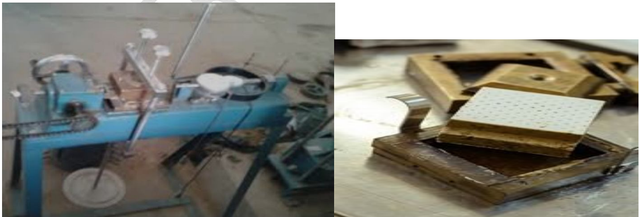
Figure 7.0: Shear box set-up
