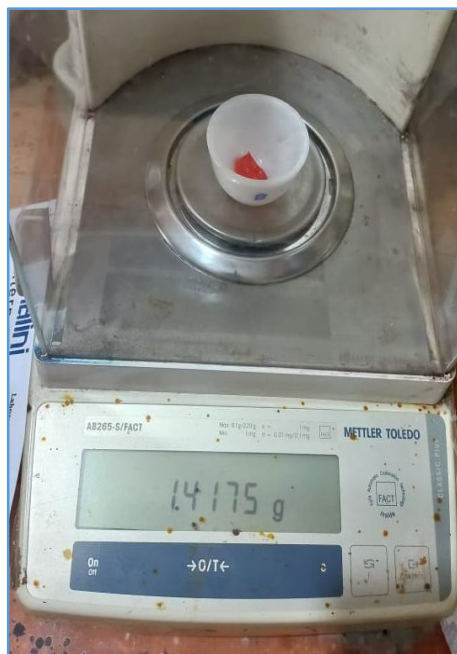
Figure 1 : Dentifrice dispensed in a teflon crucible and measured on a digital meter
