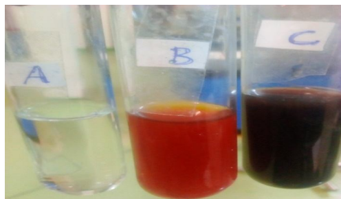
Fig. 12. Visual indication of synthesized AgNPs: A) 4mM AgNO 3 solution (colorless) B) aqueous extract of Coffea Arabica leaves (yellowish brown) C) synthesized AgNO 3 (deep brown)
