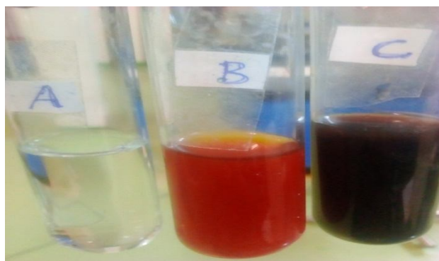
Fig. 12. Visual indication of synthesized AgNPs: A) 4mM AgNO 3 solution (colorless) B) aqueous extract of Coffea Arabica leaves (yellowish brown) C) synthesized AgNO 3 (deep brown)
