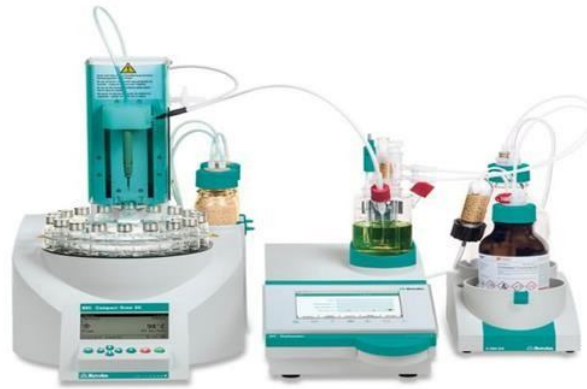
FIG. 2 Karl Fisher Titration of the instrument [10]
