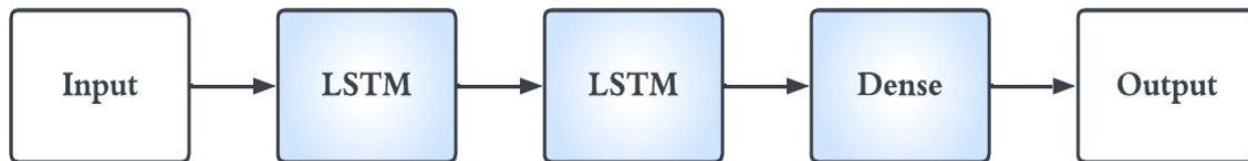
Fig. 3: The stacked long short-term memory (LSTM) architecture
