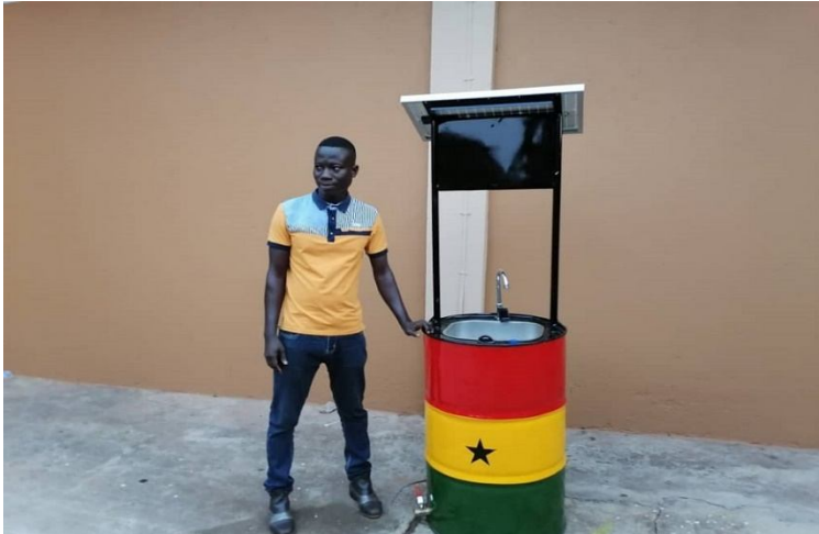
Figure1: A Solar-powered hand washing sink
