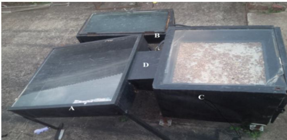
Figure 1. The solar dryer. A – Flat Plate Solar Collector B – Parabolic Solar Collector (Heat Storage Chamber) C – Drying Chamber D – Air duct Unit (Fagunwa et al., 2019).
