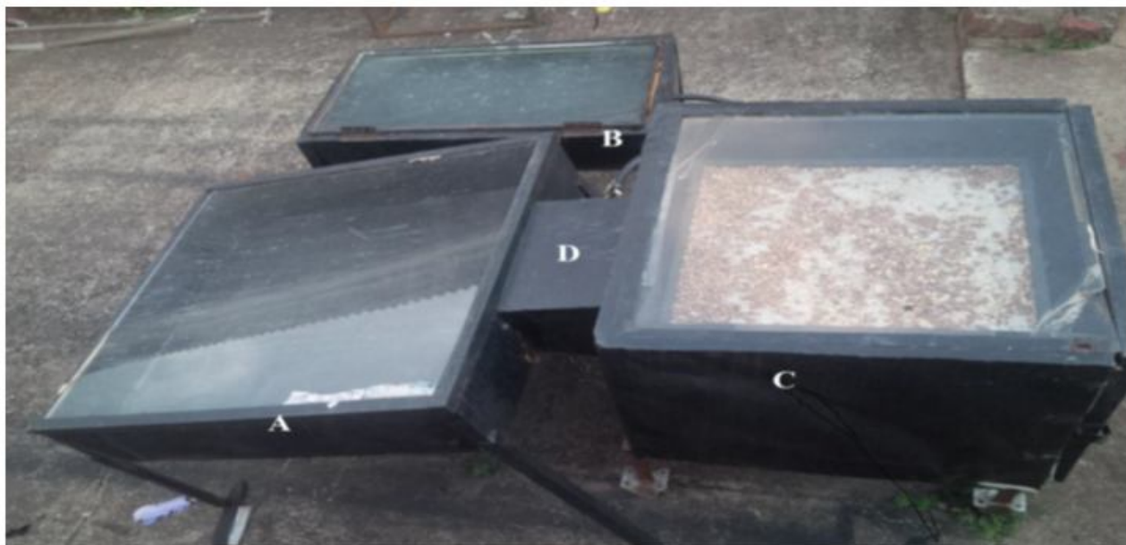
Figure 1. The solar dryer. A – Flat Plate Solar Collector B – Parabolic Solar Collector (Heat Storage Chamber) C – Drying Chamber D – Air duct Unit (Fagunwa et al., 2019).
