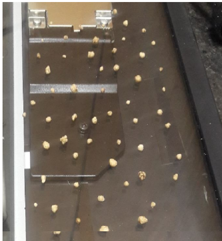
Figure 1. Shape and size determination of DAP granules using Grain size and shape properties software
