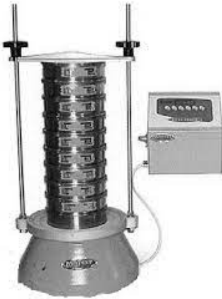
Fig. 1. Schematic of a typical mechanical sieve shaker [7].
