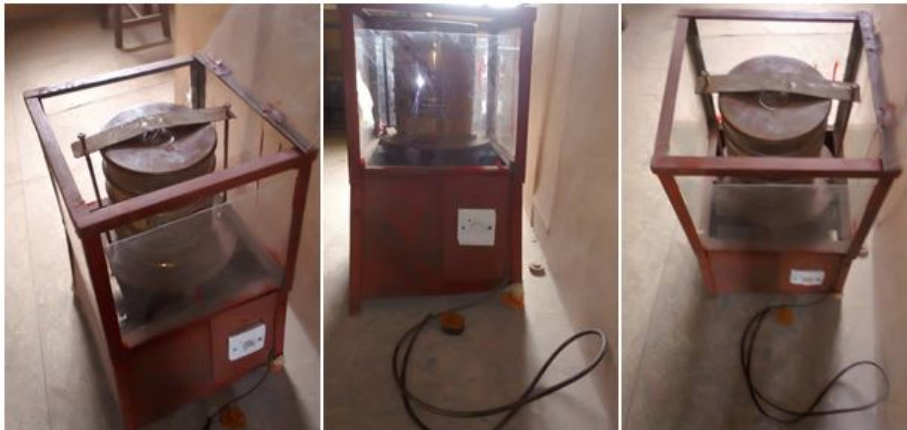
Fig. 4. Schematic of the fabricated mechanical sieve shaker
