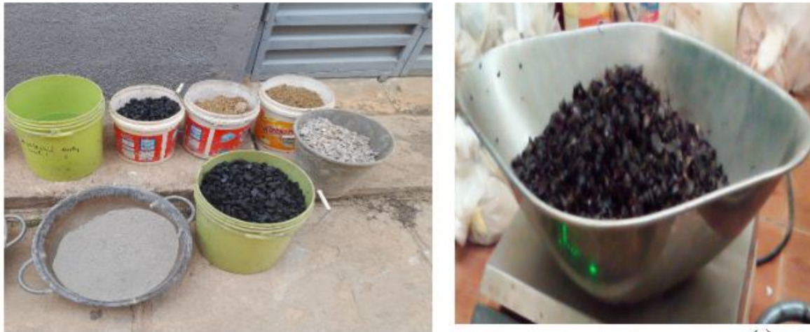
Fig. 1 (a) Cement, sand, tire and crushed granite aggregates (b) PKS aggregates
