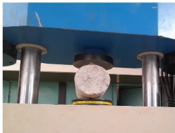
Fig 3. Split tensile test
