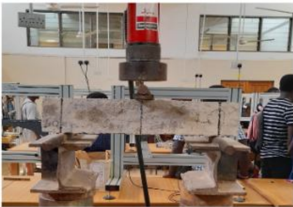
Fig. 2- Modulus of rupture test
