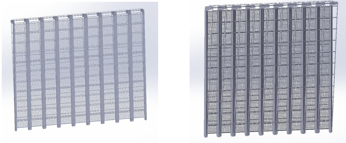
Fig.5. Front view of algae interception mechanism Fig.6. Reverse view of algae interception mechanism
